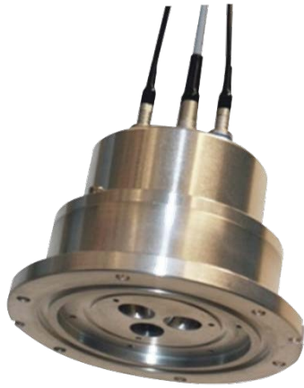
Figure 18: Picture of the experimental three axes test system which has been mounted below a car.
