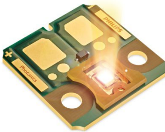
Figure 3: Photograph of an illumination product. The high power VCSEL array is emphasized by the illustrated emission cone.
